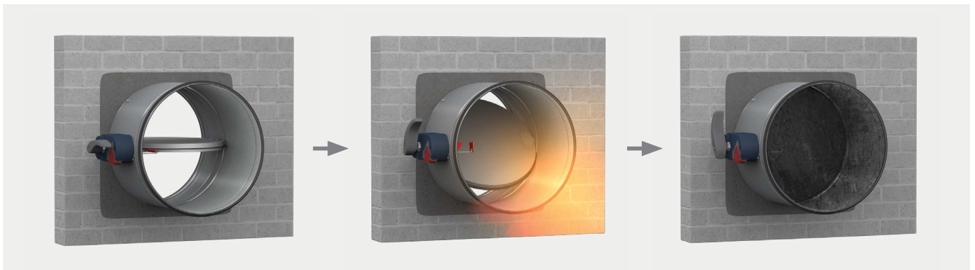
Operation of the fire damper
